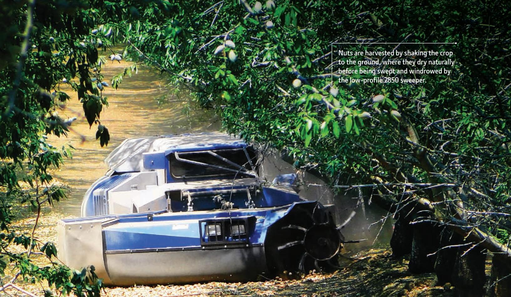
To maneuver beneath low-lying limbs, Weiss McNair of Chico, California, offers the 2850, a low-profile self-propelled sweeper with a cab height measuring a mere 1.37 meters (54 inches) high — the shortest Final Tier 4 sweeper in its class.
