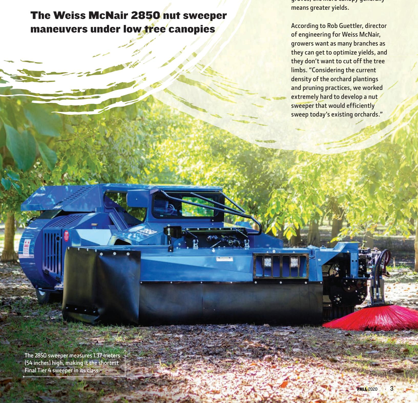
The 2850 sweeper measures 1.37 meters (54 inches) high, making it the shortest Final Tier 4 sweeper in its class.
